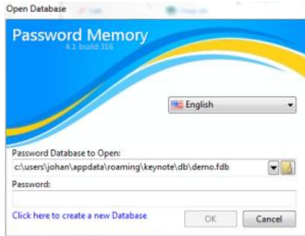
FIGURE 1. This is the Open Database dialog where you choose the password database to open and supply the password to open it. New databases can also be created by clicking the link labeled “Click here to create a new Database”.
